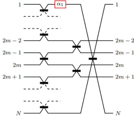
Figure 1. Interferometer design with two layers of beam splitters, proposed in [Pont22] for estimating the coefficient of genuine multiphoton indistinguishability from the visibility obtained when varying the phase  $\alpha_1$ , using preparation and detection of single photons in odd-numbered inputs and outputs.
