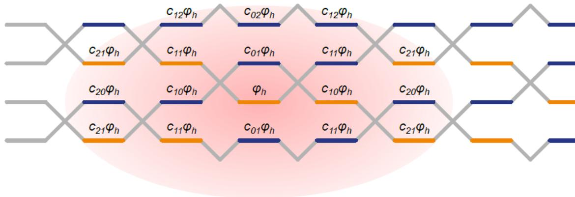
Figure 6 Illustration of thermal cross-talk on neighbouring waveguide sections in a quantum photonic processor (QPP).
