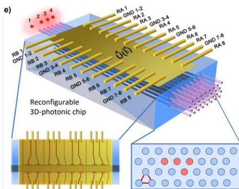
Figure 3. 3D laser-written multimode interferometer demonstrated in boson sampling experiments reported in [Hoch22]. 16 resistors on the device's surface can be controlled to locally change the index of refraction, effectively reconfiguring this 32-mode device. Waveguides are coupled by evanescent field coupling in a triangular lattice (bottom right).
